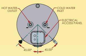
The Inlet & Outlet have Built in Heat Traps, Keeping the Heat in the Tank for Greater Efficiency
