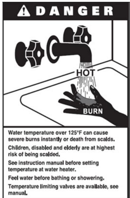
To protect against injury, install a mixing valve in the water system. This valve will reduce point of use discharge temperatures by mixing cold and hot water in branch supply lines. Such valves are available from your local plumbing supplier.
