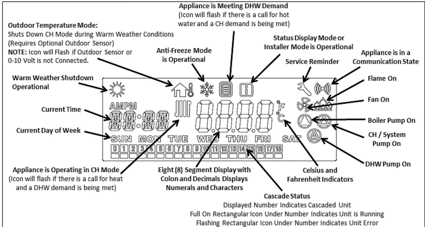
Figure 36 – LCD Display Detail
