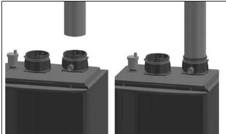
**Figure 7 – Installing the 6" Length of CPVC into the Exhaust Vent Connection**
