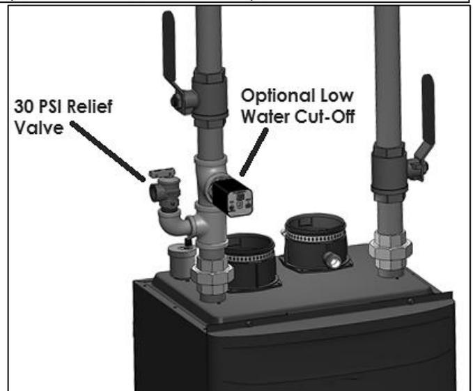
**Figure 27 – Relief Valve Details**
