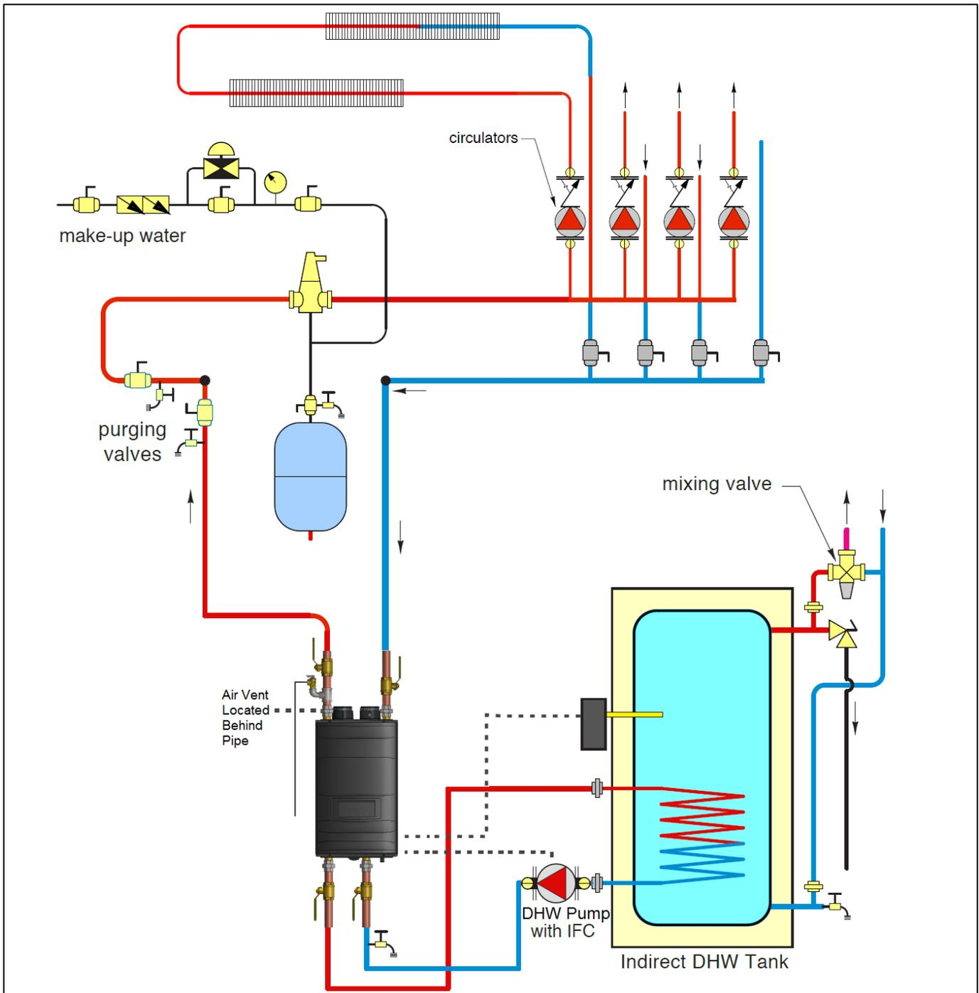
Figure 21 – Zoning with Pumps and Indirect Fired Water Heater – Direct Piping
