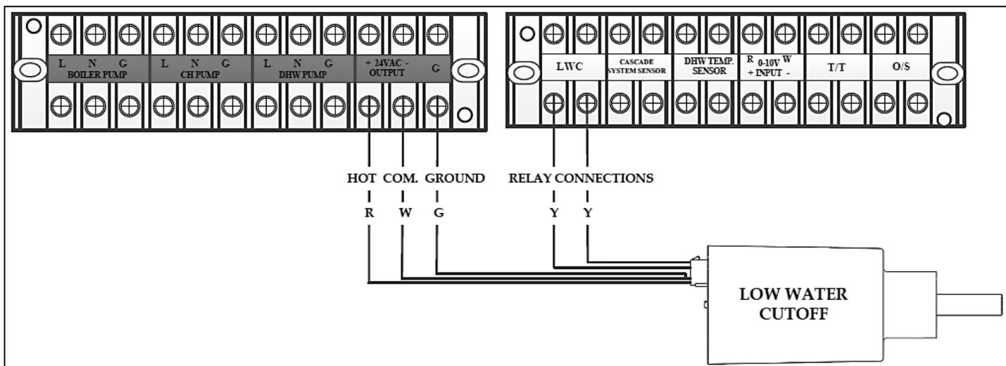
Figure 28 – Wiring External LWCO to the Boiler
