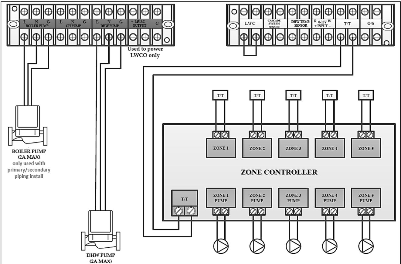
Figure 25 – Wiring – Zoning with Pumps and Indirect Water Heating
