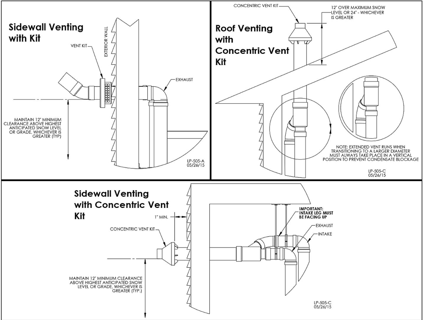
Figure 10 – Direct Vent, Vent Terminations (With Optional Kits)
