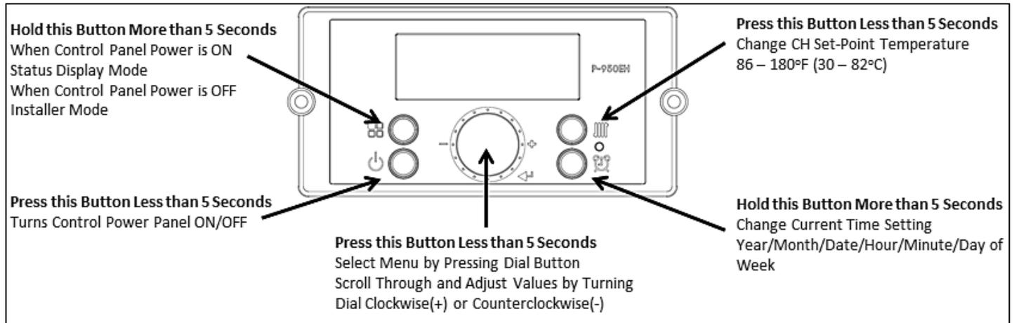
Figure 35 – Boiler Control Panel Detail
