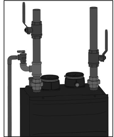
**Figure 26 – Pressure Relief Valve**
