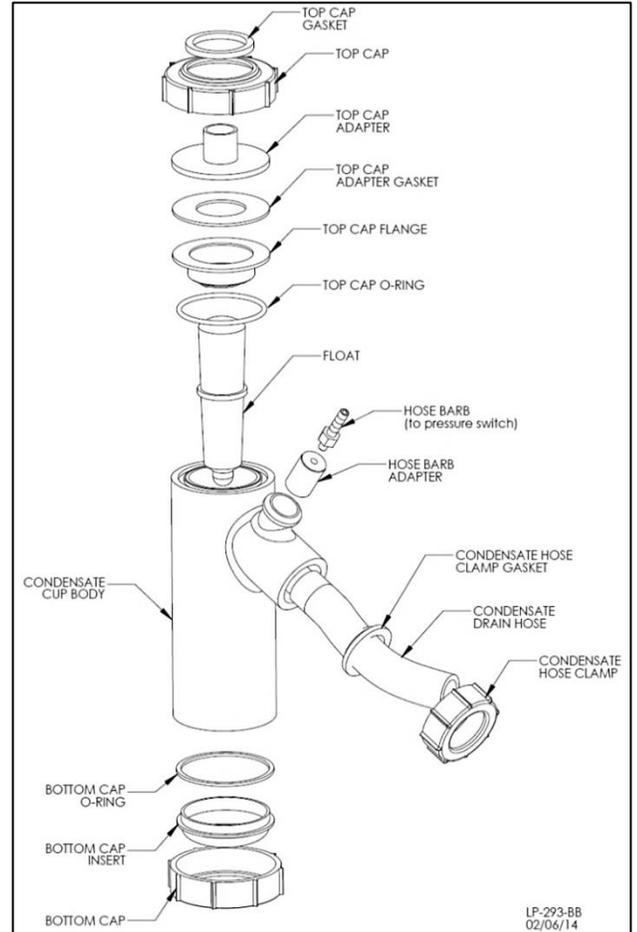
**Figure 52 – Condensate Detail**
