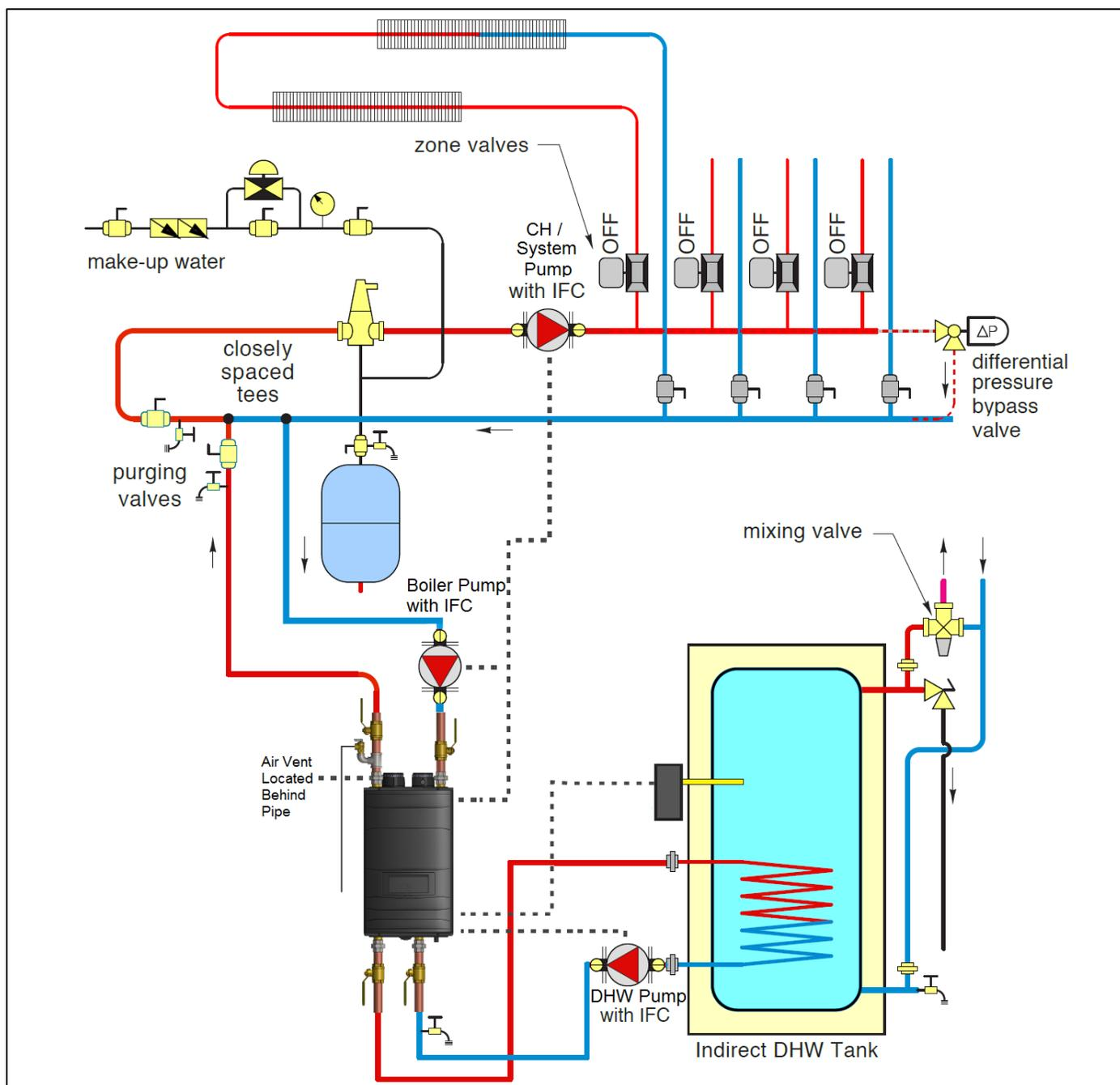
Figure 22 – Zoning with Zone Valves and Indirect Water Heating – Primary / Secondary Shown
