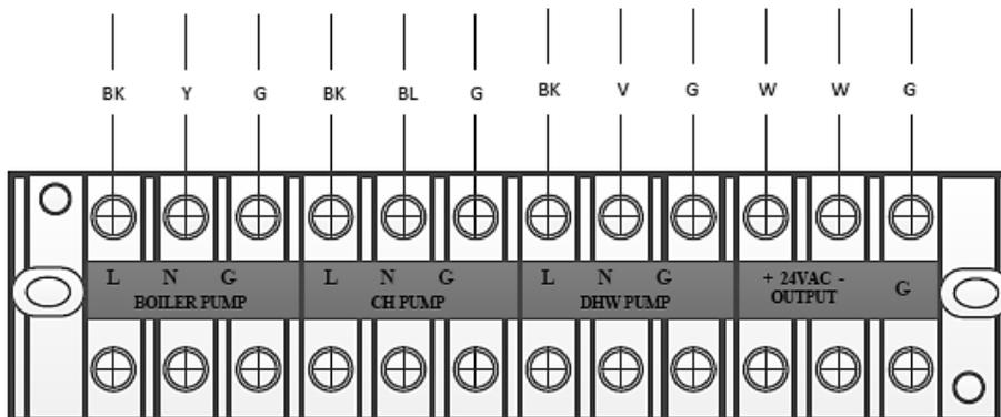
Figure 33 – Line Voltage Wiring Detail
