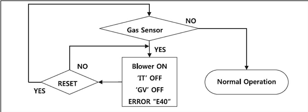
Figure 44 – Gas Detection Error Analysis Tree
