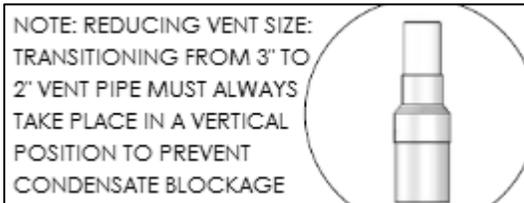
**Figure 8 – Transitioning from 3" to 2" Vent Pipe**
