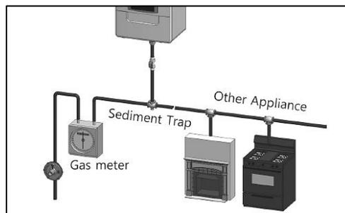
**Figure 17 – Natural Gas Piping Installation – NOTE: Capacity to be Not Less than Total Capacity of Connected Boilers**
