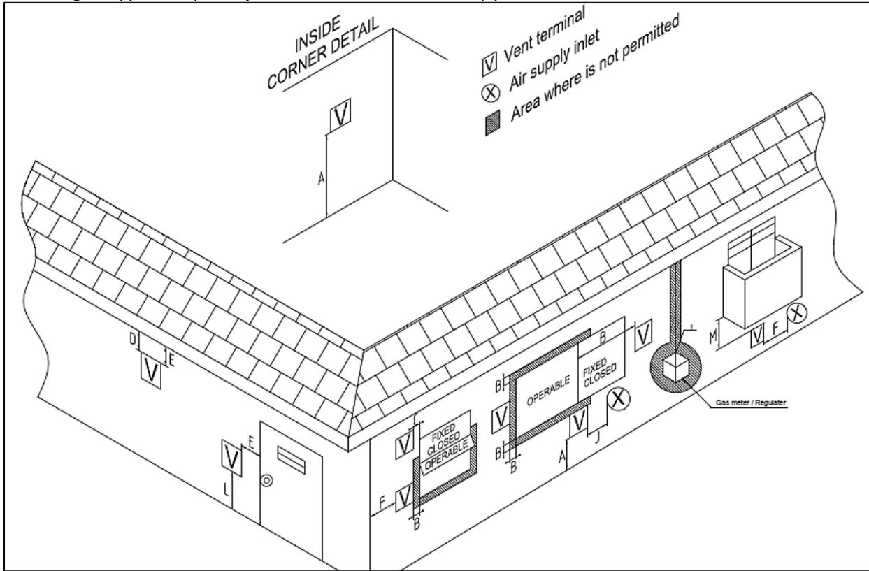
Figure 6 – Vent Termination Detail
