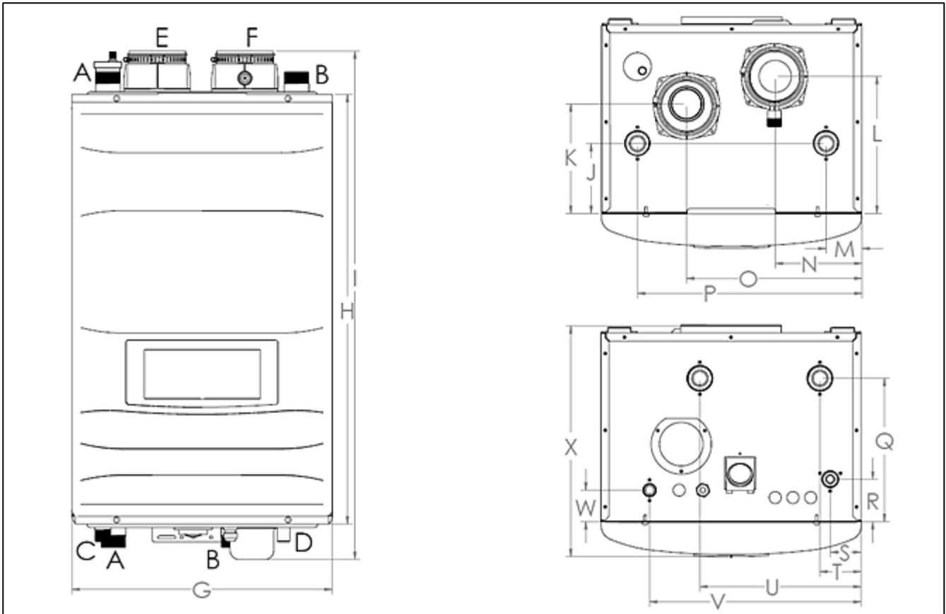
Figure 1 – UFT Specifications and Dimensions
